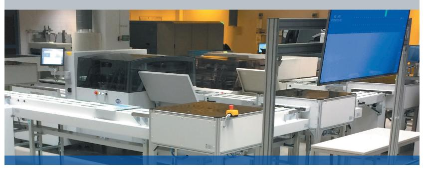
In the **NELAVCP***evolution*, video cameras detect the exposed register marks on the imaged offset plates. Thanks to its state-of-the-art image processing and positioning units, each printing plates is brought into a register-true position that corresponds with the image. When properly aligned, the printing plates are punched and bent in one cycle before they are carefully placed into the customizable stacking station.
